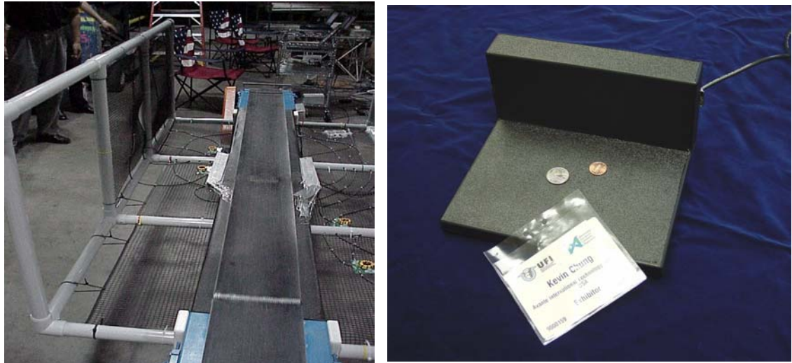
Figure 5a: The patent-pending (allowed) antenna array portal on the left was designed to have an open top [3]. This design permits the large and taller articles to be tracked as long as the tag is placed at below 30-in height. It has been proven in official FAA test to track bags with tags in all position within the portal and random orientation at 8 feet/second.
