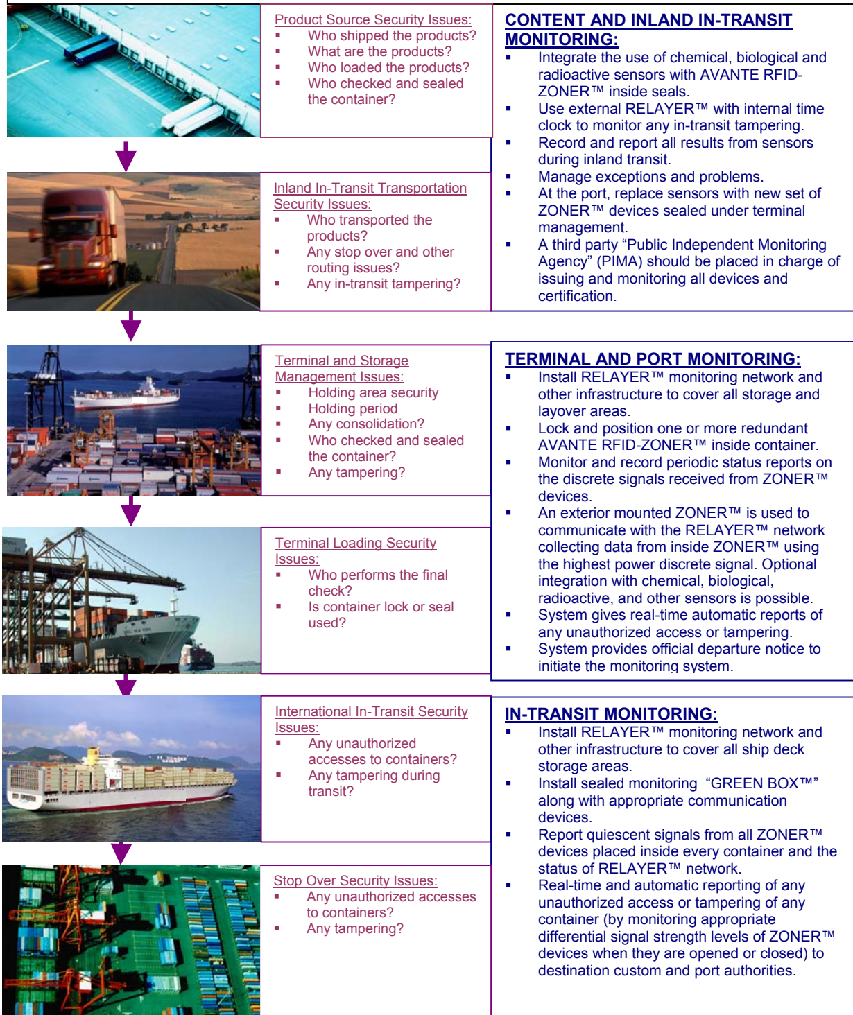
Figure 5: A pictorial representation of a secure supply chain management system with 100% end-to-end visibility of containers that are individually monitored and tracked in real-time.
